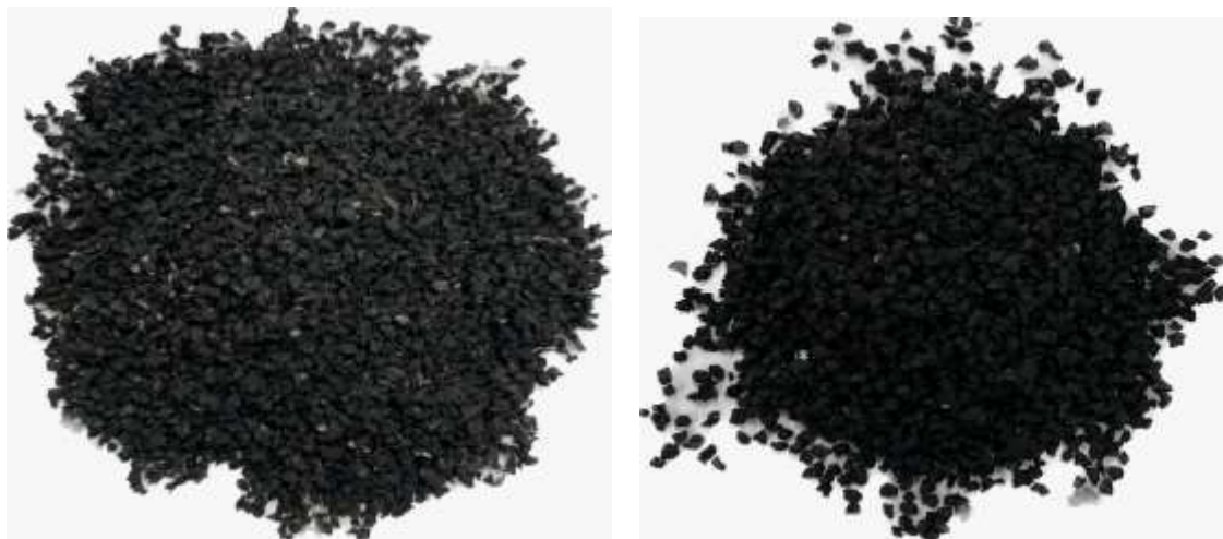
Figure 2.2: The main types of recycled rubber used in the manufacture of cement products are (a) hard crumb rubber and (b) soft crumb rubber [3]
